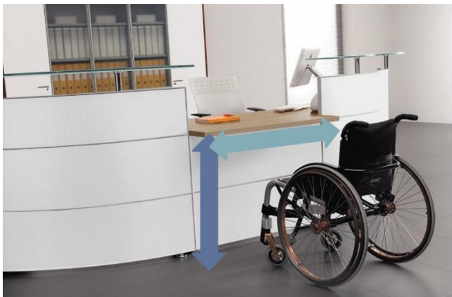
A usable reception counter is at least 36" wide and no more than 36" high
